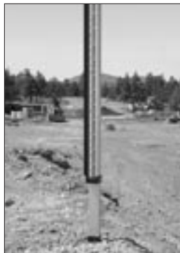
Rod extension fully collapsed
